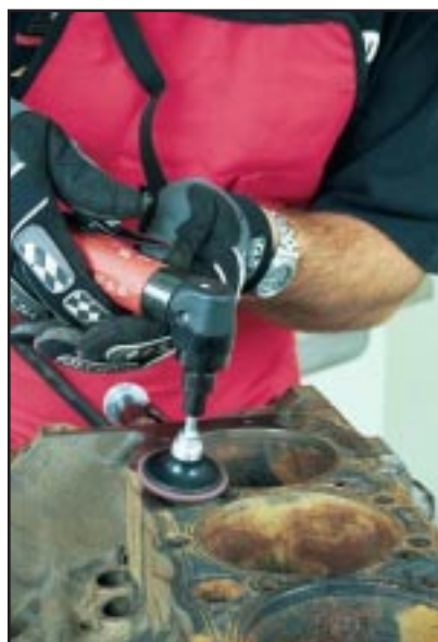
The key to good work with power-driven abrasive products is to control the grinder with both hands and let the rotating action of the abrasive do the work. Use only limited downward pressure, if any at all.
