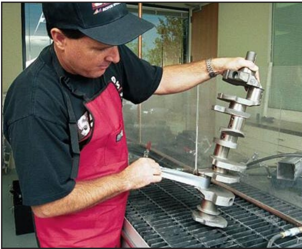
Duct tape greatly decreases the threat of a nicked journal if you catch a bearing journal with the tool.
