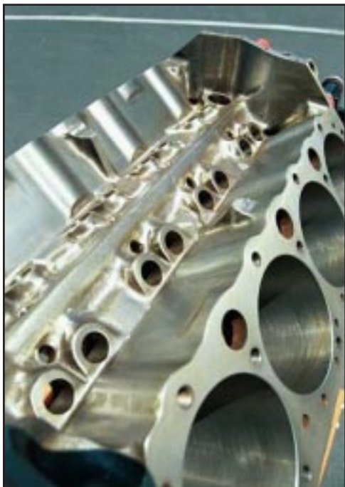
Our finished demo block shows the comprehensive deburring job one can do with the Standard Abrasives Block Prep Kit.
