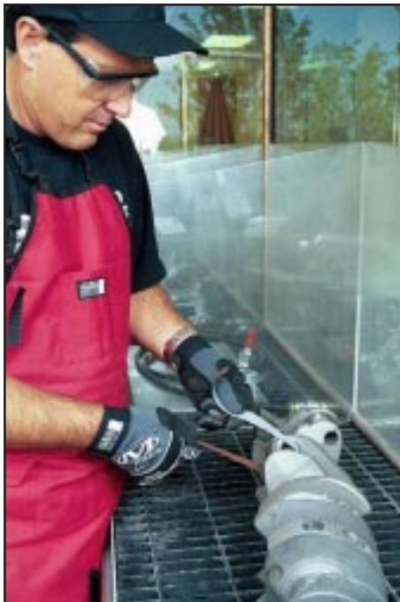
In the unfortunate event you do damage a crankshaft journal or thrust surface, the Block Prep Kit's Handy Roll will usually repair the problem.
