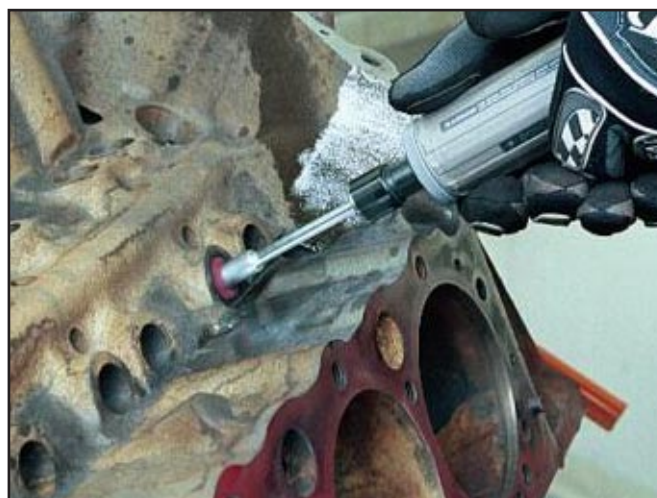
In block preparation work, the main application of Cross-Buffs™ is the surface preparation of the valve lifter bores.
