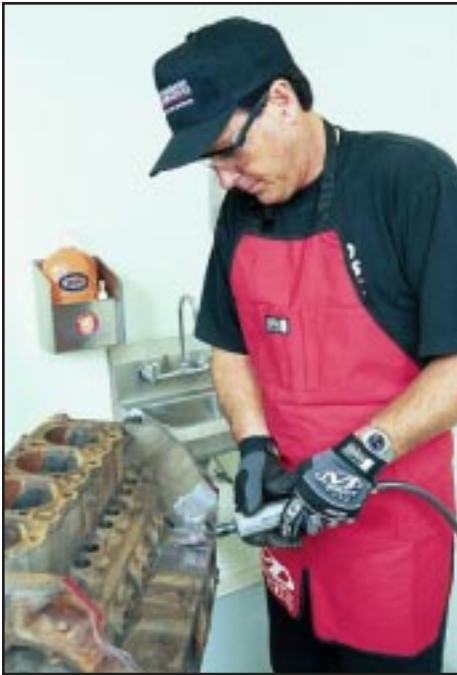
After the oil hole work, depending on the surface, use tapered or straight cartridge rolls, to deburr and smooth valley areas.
