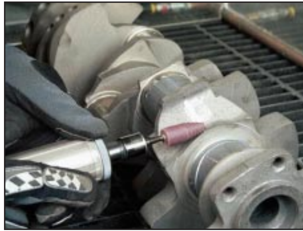
Sharp edges just outside the bearing journals must be approached with care using a tapered Cartridge Roll. Do not heavily radius these edges. In some cases, such as this Chevrolet crank, you may be working near the crank's thrust bearing surface. Take care not to nick the thrust surface.
